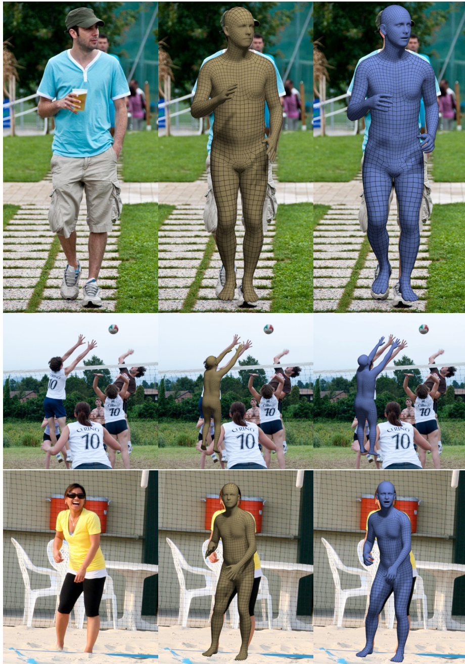
Fig. 20: Comparison of ExPose with the state-of-the-art body regression method: 1. RGB image, 2. SPIN [5], 3. ExPose. Our proposed method produces 3D body pose and shape results on par with SPIN [5] and captures more details for the hands and face.
