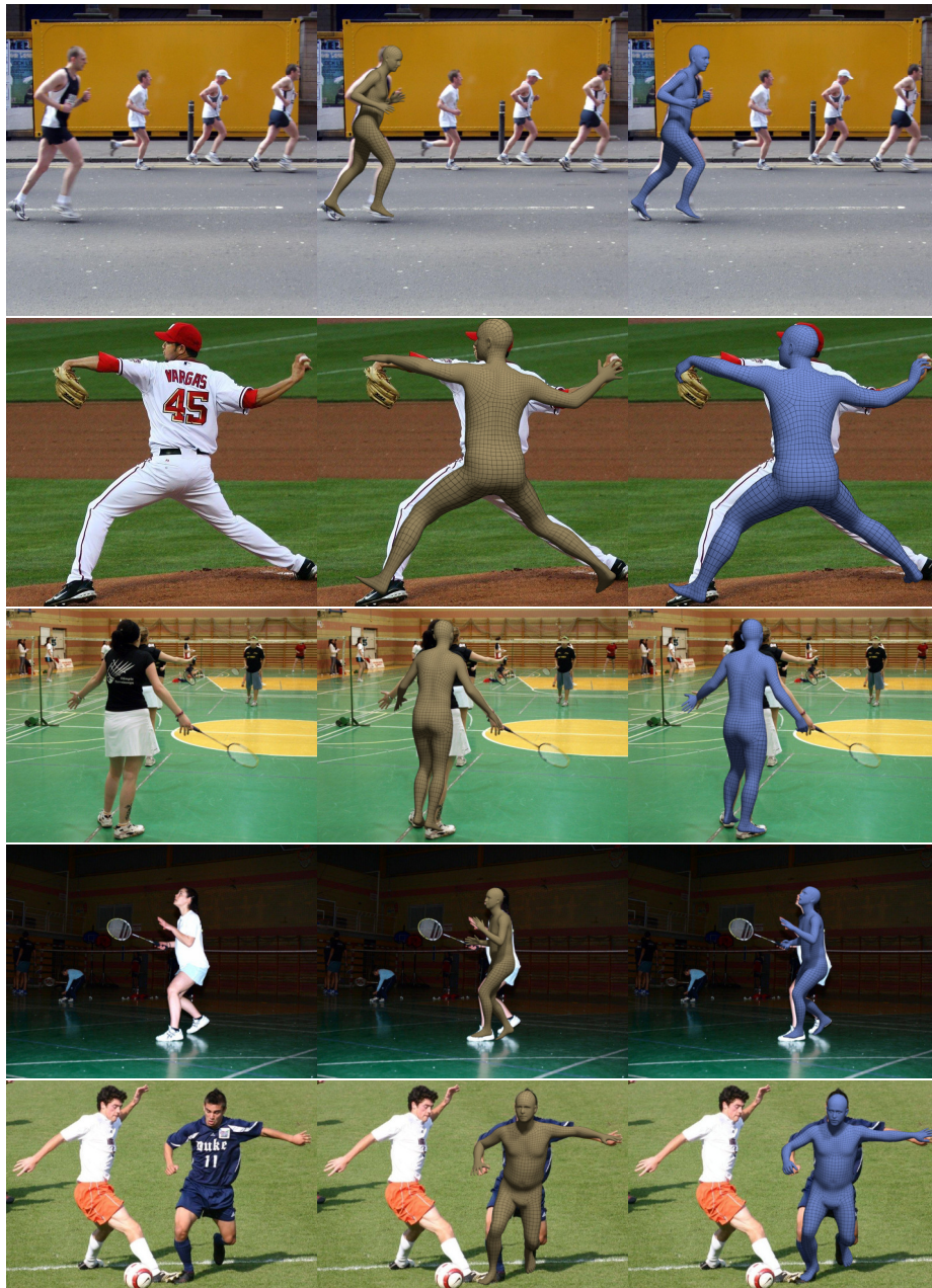
Fig. 11: Comparison of ExPose with the state-of-the-art body regression method: 1. RGB image, 2. SPIN [5], 3. ExPose. Our proposed method produces 3D body pose and shape results on par with SPIN [5] and captures more details for the hands and face.
