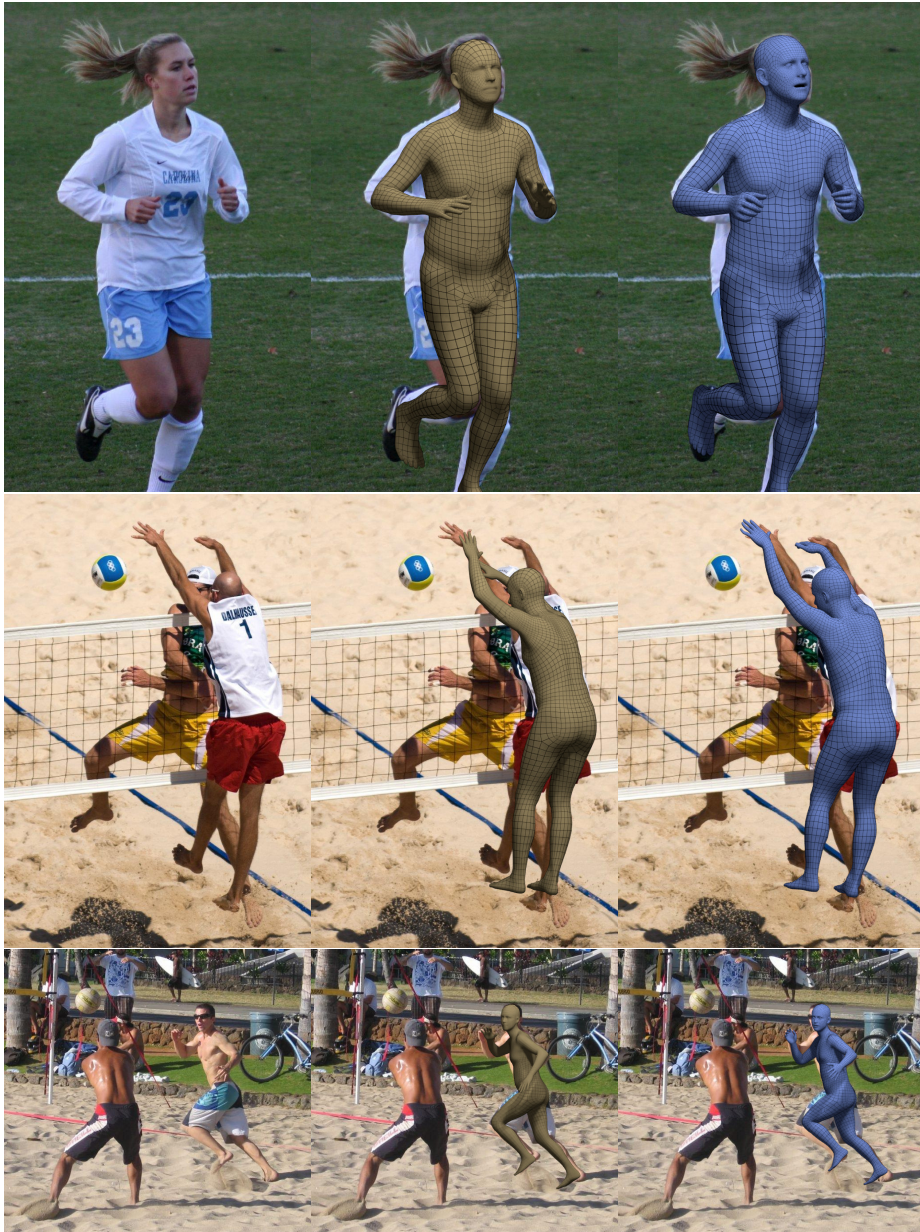
Fig. 19: Comparison of ExPose with the state-of-the-art body regression method: 1. RGB image, 2. SPIN [5], 3. ExPose. Our proposed method produces 3D body pose and shape results on par with SPIN [5] and captures more details for the hands and face.
