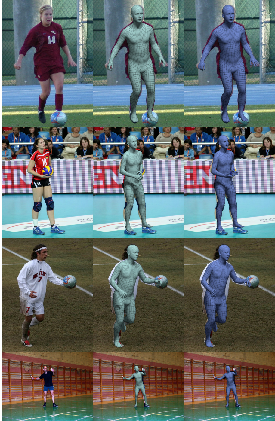
Fig. 9: Left : The input image. Middle : Naive regression from a body crop. Right : ExPose. The attention mechanism helps capture detailed hand articulation and facial expression.
